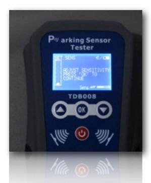
MEASURE THE FIRST PARKING SENSOR AND PRESS OK WHEN COMPLETE
