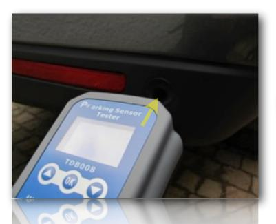
SELECT THE REQUIRED TEST AND POINT THE TDB008 SENSOR PICK UP TOWARDS THE PARKING SENSOR
