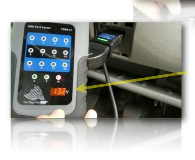
VOLTAGE READING WITH TDB013 CONNECTED
