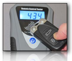
IMPORTANT NOTE : If you receive erratic or incorrect frequency readings, ensure the device is away from Mobile Phones, Wireless internet, Bluetooth devices etc. These devices work on similar frequencies to some of the remote controls and therefore it is important that they are not in close proximity while the test is performed.
